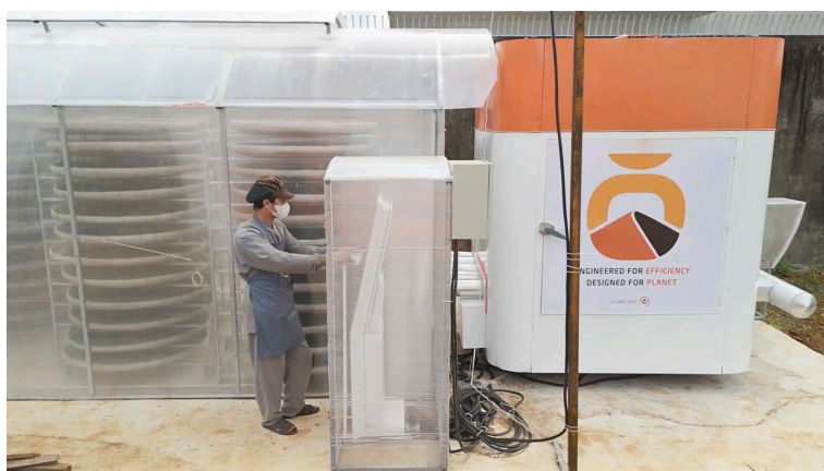
Fig 9. Application of sand battery to dry tea in greenhouse
